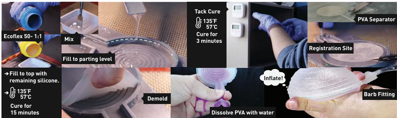
**Figure 4.** Bladder Fabrication Process. A single batch of silicone is prepared to fill a mold up to the parting level and speed cured to a tack state. A 3D-printed PVA separator is laid on the base layer, using a registration site to help anchor and align the element. The remaining silicone is poured and speed cured. Once demolded, the bladder is inflated with warm water to dissolve the PVA and the resulting bladder is inflated.
