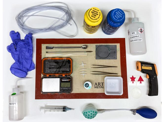
Figure 3. Materials, tools, and equipment used in bladder fabrication and testing. From bottom left, clockwise, moving inward: A water bottle, nitrile gloves, air tube, EcoFlex-50 silicone, isopropyl alcohol, an infrared heat gun, vinyl, polyvinyl acetate, a inflation bulb with valve, a syringe, a scale, glass rods, metal spatulas, molds, tweezers, antistatic weigh boats, silicone colorant, barbed airtube connectors. Not pictured: an FDM 3D printer, an incubator, and vinyl cutter.
