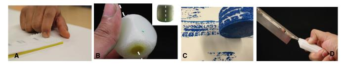
Figure 7. (a) A fan control board. A multi-button pattern is attached to a capacitive layer (bottom) and a raised texture-enchanced surface is placed to give the interface tactile cues and affordances. (b) A weighted die. Acrylic medium is pipetted into an axial chamber. (top) The die backlit. (c) A printmaking wheel with texture, compliance, and weight. (d) A blade handle with additional pressure cues to indicate correct finger placement.
