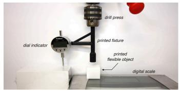
Figure 8. Our compliance testing setup measured force with respect to applied displacement. The drill press was manually operated.
