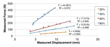
Figure 9. Linear regressions for various percentages of infill and their corresponding compliance. Spring rates require a y-intercept at 0.
