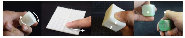
Figure 1. Example objects created with HapticPrint. External and Internal tools allow users to easily add tactility, flexibility, and weight to objects.
