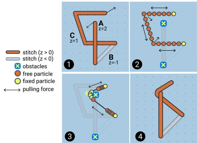
Figure 4: Pulling a thread. (1) Embroidery geometries are encoded as a set of stacked stitches; (2) stitch C is simulated as a linked particle system; the ingress and egress of stitches above C are set as obstacles - a pulling force is applied on the particles; (3) as particles collide with obstacles, they become fixed; the simulation runs until the change in stitch length is negligible; (4) stitch C is constrained by stitch A.
