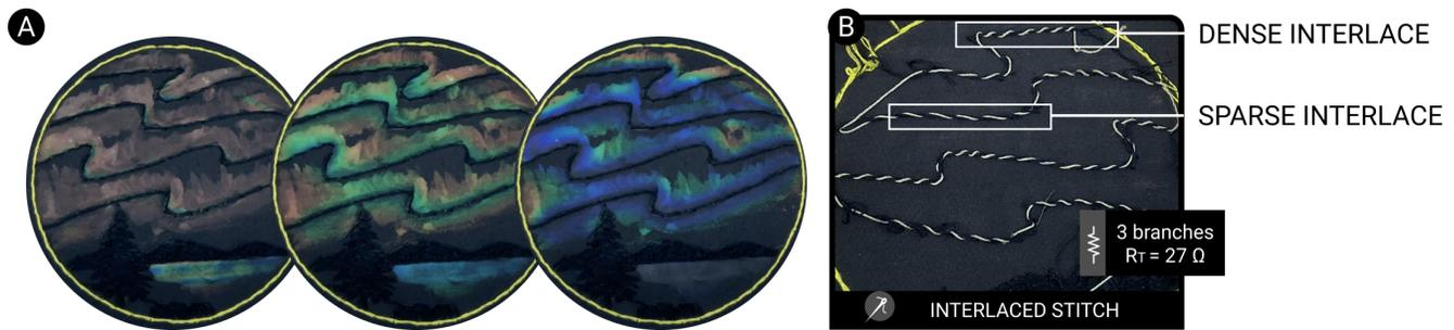
**Figure 7: Aurora Borealis. (A) A heat-variant LCTD produces non-uniform regions of heat to activate the larger spectrum of liquid crystal colors over time; (B) a conductive thread is interlaced on the structure of a regular thread backstitch to reduce thread visibility.**
