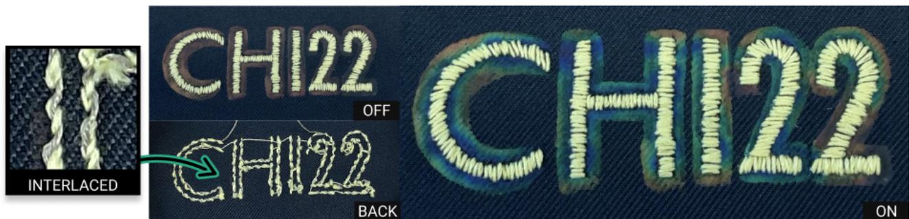
**Figure 1:** A hand-embroidered Liquid Crystal Textile Display (LCTD) is created by interlacing a conductive thread along the back of a satin stitch. When powered, the thread acts as a resistive heater causing painted liquid crystal to change colors.
