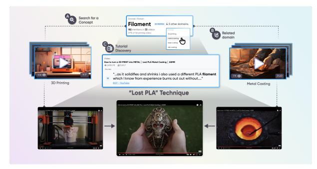
Figure 4: The process of discovering the "Lost PLA" technique, by Robinson Foundry, in which a PLA scuplture is coated in a ceramic mold and subsequently burned away with molten metal.
